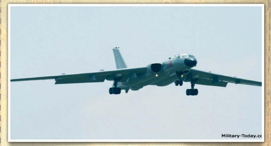
The H-6K can carry under its wing pylons six conventional or nuclear armed CJ-10A cruise missiles with 2,200 KM range. Although the H-6 was first domestically produced in 1968, this upgraded version, using composite materials, modern avionics and a powerful radar, first entered service only in October 2009.
