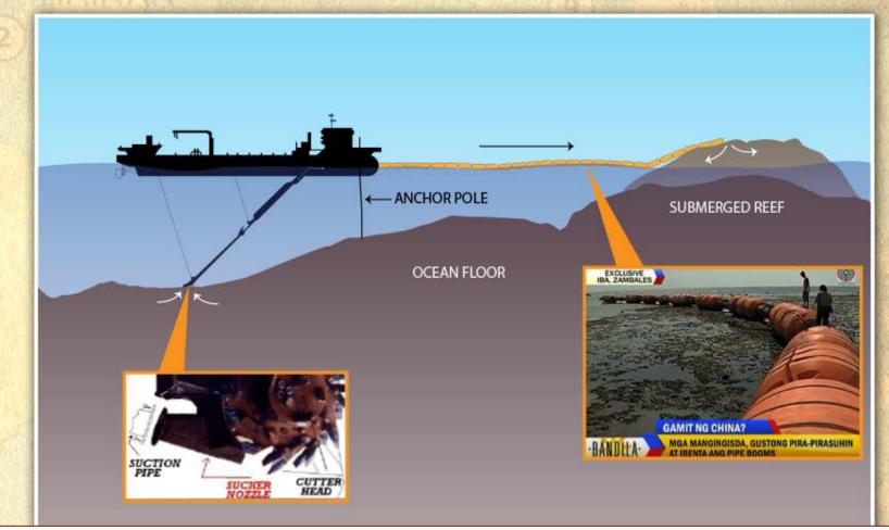
Coral reef and hard sediment on the seabed are pulverized by the rotating cutter. Pulverized materials are sucked into the ship. Pulverized materials are transported by pressure through a floating pipe. Pulverized materials are deposited on the rim of the reef.
