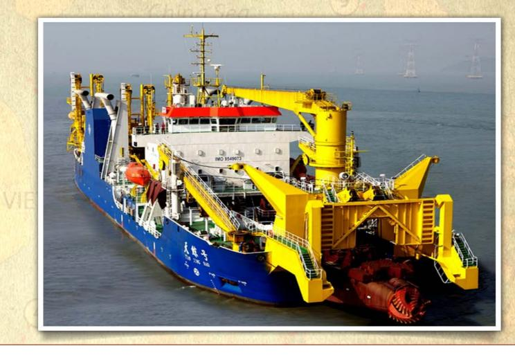
The *Tiang Jing Hao* dredger, a 127 meter-long seagoing cutter suction dredger designed by the German engineering company Vosta LMG. At 6,017 gross tons, this dredger is the largest in Asia. China has dozens of dredgers in the Spratlys.
